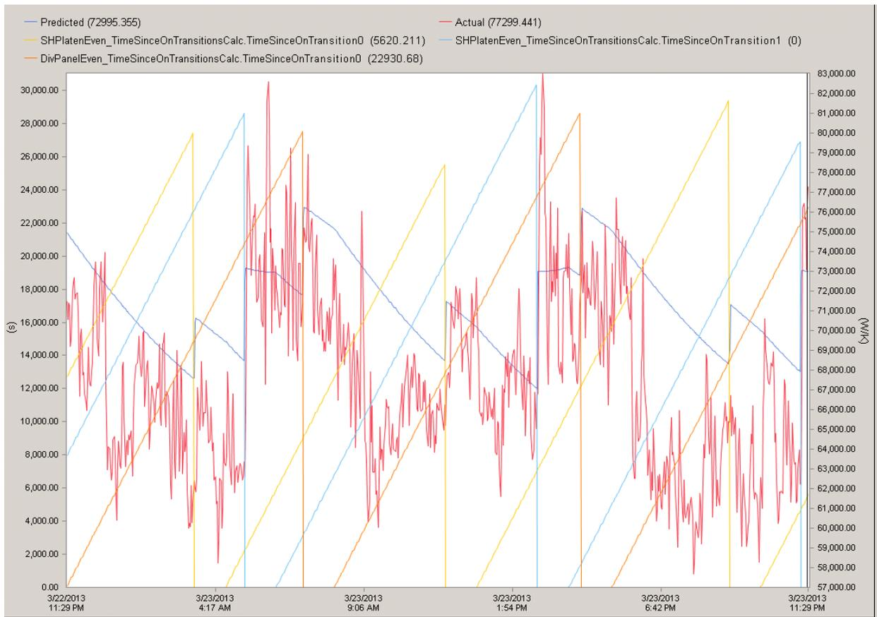
**Figure 3:** Heat transfer coefficient for the division panel section shown in red for a one day period. The yellow, light blue and orange lines show the time since last activation for three blowers that affect the Division Panel section. (When a sootblower is activated, the time since value drops to zero.) The navy blue line shows a neural network model prediction of the change in heat transfer coefficient.
