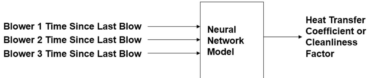
**Figure 2:** Neural network model for predicting the heat transfer coefficient or cleanliness factor. In this case, the neural network model uses the time since the last blow of the sootblowers that affect the heat transfer surface of interest.
