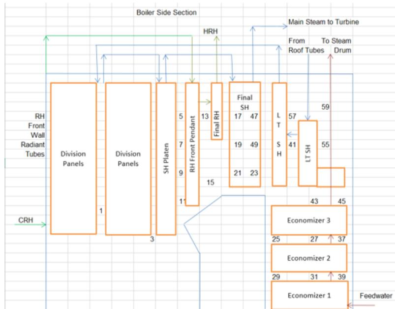
**Figure 1:** Boiler side section view of the heat transfer surfaces (after the furnace and before the air preheater) at our demonstration site. The identification number of each of the sootblowers is also shown.
