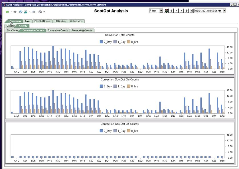
One of many analysis tools provided by SootOpt, the counts bar charts show actuation statistics over different time periods for each sootblowing device in a selected boiler area. This information helps build an understanding of baseline activity and identify changing cleaning patterns.
